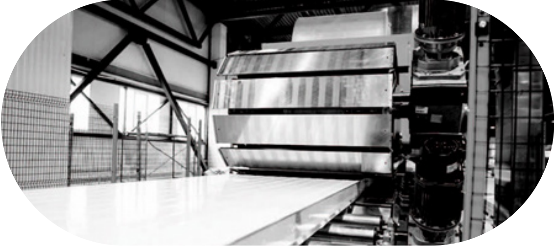
Image 2. A section of continuous line by Pu.Ma, Italy, installed in PH Insulation manufacturing facility.
