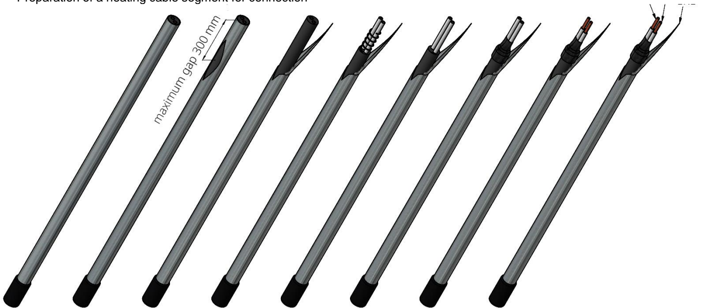
Figure 11. Preparation of a heating cable segment for connection
