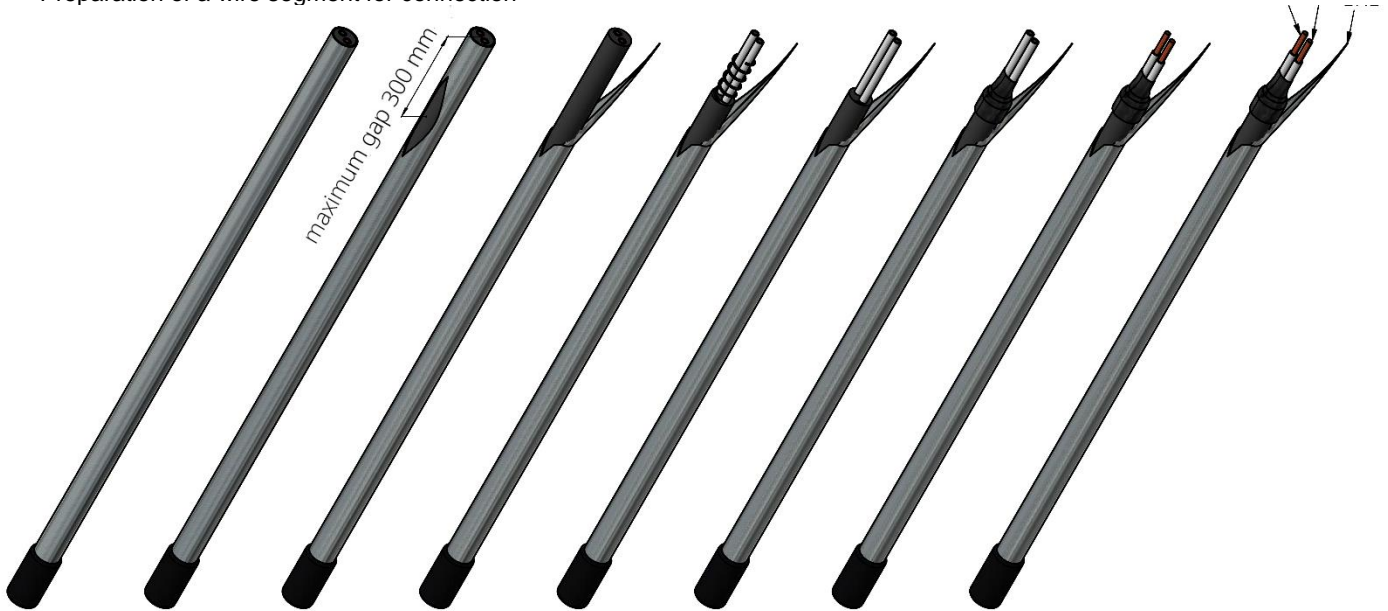
Figure 9. Preparation of a wire segment for connection
