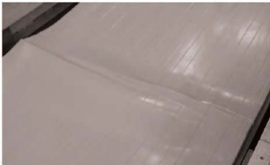
Figure 15. Forming of a fold on the sandwich panel's surface at the compression of the upper layer.
