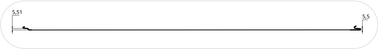
Diagram 7. Profiles of the exterior surface of PWT SF sandwich panels, dimensions are indicated in mm
