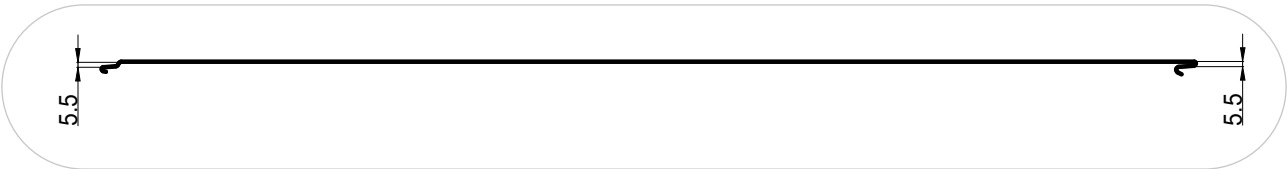
Diagram 6. Profiles of the exterior surface of PWT Z sandwich panels, dimensions are indicated in mm
