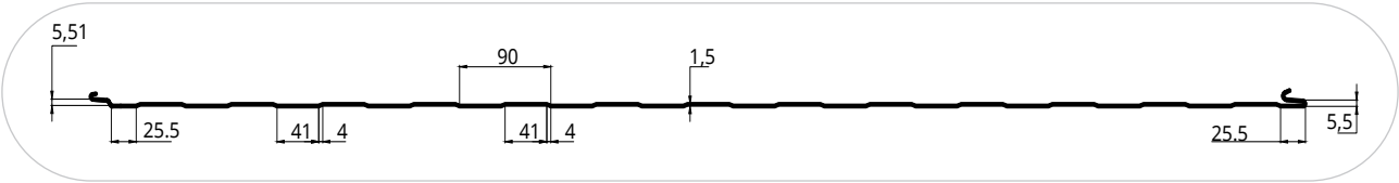
Diagram 6. Profiles of the exterior surface of PWT Z sandwich panels, dimensions are indicated in mm
